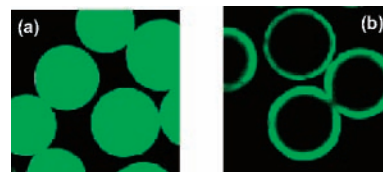
Figure 2. Cross-sectional images of the FITC-coupled resins viewed through a confocal microscope: (a) TentaGel resin (0.30 mmol NH 2 /g); (b) HiCore resin (0.32 mmol NH 2 /g).
